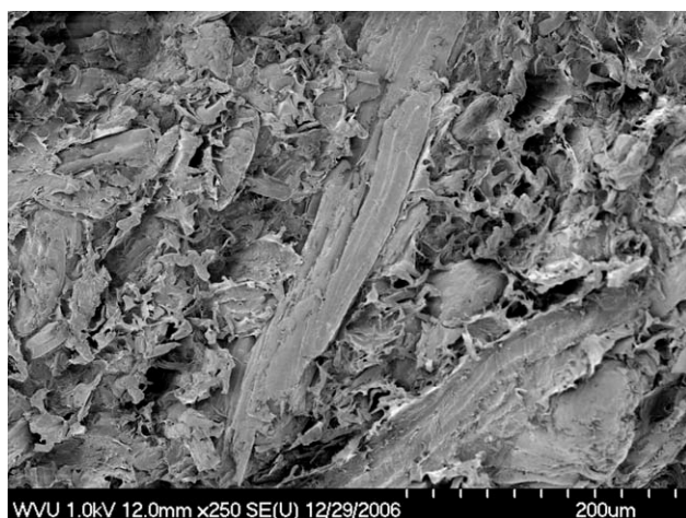
Figure 8. Tensile fracture surface of 50 wt % wood WPCs containing 1 wt % of SEBS-g-MA.
